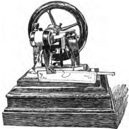
ELIAS HOWE'S ORIGINAL MODEL OF THE SEWING MACHINE.
